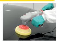
Attach 3M<sup>™</sup> High Gloss Polishing Pad (50488) to rotary polisher and start up machine, move across panel until high shine is achieved.
