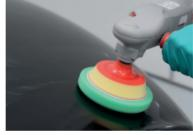
Place pad onto panel and start up rotary polisher. Work a small area at a time, re-applying compound when moving to a new area.
