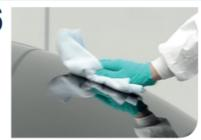
Finally remove liquid residue using a 3M<sup>™</sup> Perfect-It III<sup>™</sup> Ultrafina High Performance Cloth.
