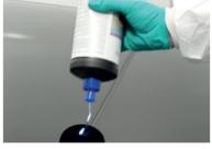
Shake bottle and apply 3M<sup>™</sup> Perfect-It III<sup>™</sup> Ultrafina SE (50383) to the vehicle, aiming to work half a square metre at a time.
